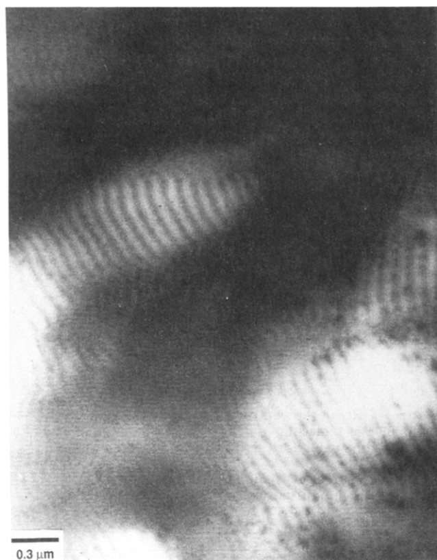
Figure 5. Electron photomicrograph of the neat triblock copolymer.
